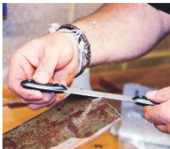
▲ The grips prove useful for honing larger blades such as this adze
